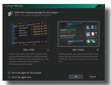
15. Click on the Add Event button, key down, and finally, left. A new dialogue box will appear asking if the software should run in visual or code mode. Here select visual to build with blocks and check Don't Ask Again for this Project. There is now an event for when the left key is down but no action takes place when this happens... the event needs an action on the event will do nothing.
